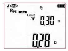
Positive visual inspection result. The tester will automatically run the subsequent tests: RPE.
