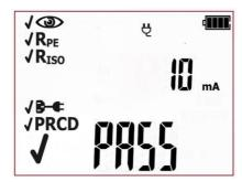
Correct result. The result of each single test of the sequence is positive. Green LEDs of PASS indication are on.
