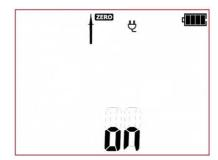
The compensation value has been measured. M is displayed on the screen, along with the permanent symbol. After 3 seconds the tester returns measurement mode. The active test lead compensation is indicated by ZERO icon displayed on screen during the tests of R<sub>PE</sub> (200mA, 10A) and CL I autotests. compensation The sistance will be taken into account then displaying test results of Rpf.
