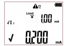
Correct result. The value of leakage current is below the set limit. Green LEDs of PASS indication are on.
