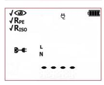
Measurement of insulation resistance has been completed. If the measurement result is negative, further measurements will not be conducted. In case of the positive test result: the tester will automatically run the subsequent tests – polarity check.
