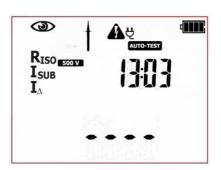
The tester is in autotest mode for Class II devices. Icons displayed on the left side represent all tests that will be performed. On the right side the current time is shown.
