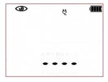
The tester is waiting for the evaluation of the device after completing visual inspection. If the measurement of the L-N circuit resistance is selected, tester will also display the result of R<sub>LN</sub> measurement. If it's not selected, then dashes will be displayed in the main screen area "----".
