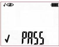
Positive visual inspection result. Green LEDs of PASS indication are on.
