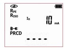
The tester is in PRCD trip time measurement mode.
