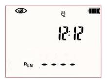
The tester is now in the preliminary test-visual inspection mode. Additionally the current time is displayed on the screen.
