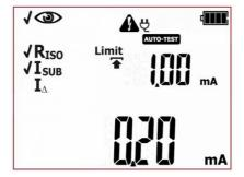
Measurement of substitite leakage current has been completed. If the measurement result is negative, further measurements will not be conducted. In case of the positive test result:
