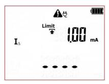
The tester is in differential leakage current measurement mode.
