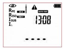
The tester is in autotest mode for Class I devices. Icons displayed on the left side represent all tests that will be performed. On the right side the current time is shown.
