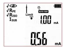
Measurement of insulation resistance has been completed. If the measurement result is negative, further measurements will not be conducted. In case of the positive test result: If the AUTO-TEST
