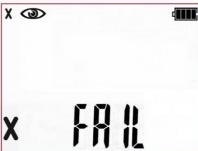
Negative visual inspection result. Red LEDs of FAIL indication are on.
