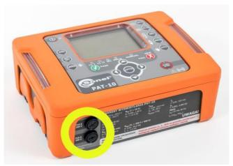
The next step is to replace the fuse with a new one and fit it together with its container back into the tester.
