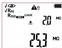
Measurement of PE protective conductor has been completed. If the measurement result is negative, further measurements will not be conducted. In case of the positive test result: the tester will automatically run the subsequent test: Riso.
