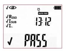
Positive test result for the tested device. The result of each single test of the sequence is positive.
