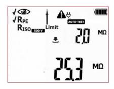
Measurement of PE protective conductor has been completed. If the measurement result is negative, further measurements will not be conducted. In case of the positive test result: If the AUTO-TEST mode is on, the tester will automatically run the subsequent test, which by default is: Riso. If the AUTO-TEST mode is off the tester will wait for the
