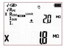
Negative test result for the tested device. One of the subsequent tests has ended with negative result - that result is displayed on screen (screen on the left, as an example, shows failed insulation resistance test). Red LEDs of FAIL indication are on.
