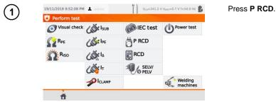
Before starting the measurement, following parameters must be set: waveform, rated RCD current and test type.
