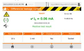
Positive test result:  $I_{\Delta} \le LIMIT$ Negative test result:  $I_{\Delta} > LIMIT$
