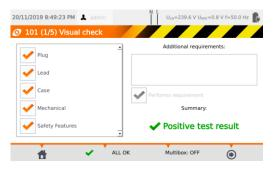
After visual test, check (or not) the corresponding boxes on the left side of the screen.
