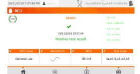
RCD must to be immediately switched on after RCD trips. Meanwhile the meter is powered from built-in rechargeable battery.
