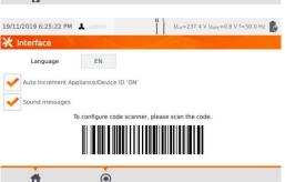
By checking the box Auto Increment Appliance/Device ID, you will enable or disable the automatic transmission of the next registration number assigned to the next device being added.
