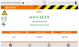
Positive test result: LOWER LIMIT ≤ I<sub>Δ</sub> ≤ UPPER LIMIT
