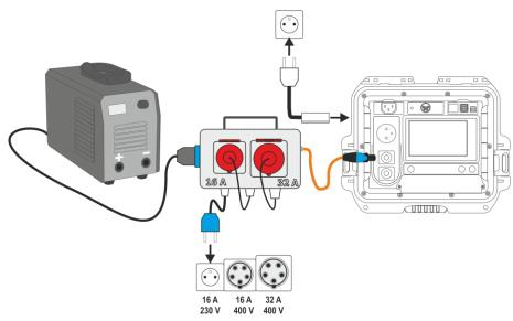
Measurement with PAT-3F-PE adapter. Connecting a 3-phase 16 A appliance.
