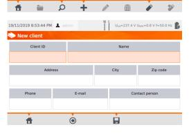
Press each field and enter client's data with on-screen keyboard. Data in red fields is mandatory.
