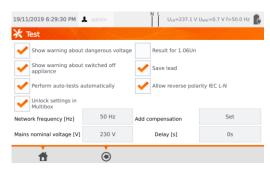
If each test is meant to be executed one after another automatically Perform auto-tests automatically option must be selected. Otherwise each test will be executed separately by pressing START button.
