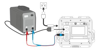
Variant with powering the welding machine directly from the mains socket.
