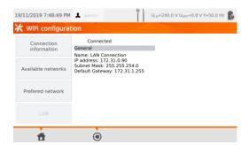
The **LAN** field displays a screen containing meter's IP in a situation, when it is connected to a LAN network.
