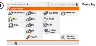
Before starting the measurement, similarly to **sec. 4.2**, following parameters must be set: **test duration**, **limit**, **polarity** and **method**.
