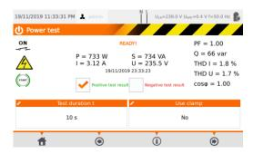
Compare the result with the technical data of the tested appliance. The assessment of the correctness of the test results can be performed by selecting the proper field in 'Positive test result' or 'Negative test result'. When saving test results in the memory, this assessment will also be saved along with the results.
