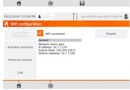
The network is saved and connection with the tester is established - connection's parameters are available.
