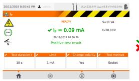
Positive test result: I<sub>P</sub> ≤ LIMIT
