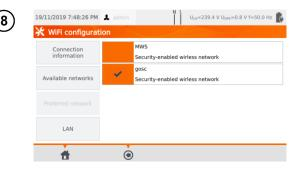
Pressing **Preferred network** enables displaying networks saved already in the tester. The network marked with is the network currently connected with the tester.
