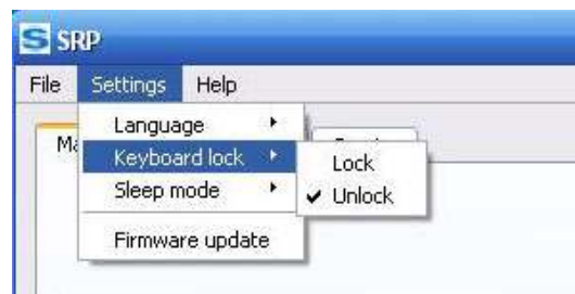
Figure 10 Locking the keypad.
