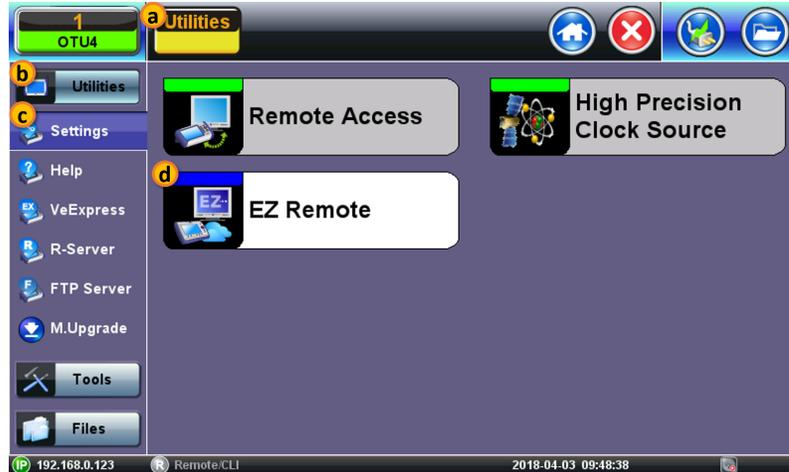
3. On the EZ Remote screen, set **EZ Remote** to **Enable**, confirm the **URL** is **ezremote.veexinc.net** (without www.), and tap on **Apply** to connect and establish a session with the EZ Remote server.
