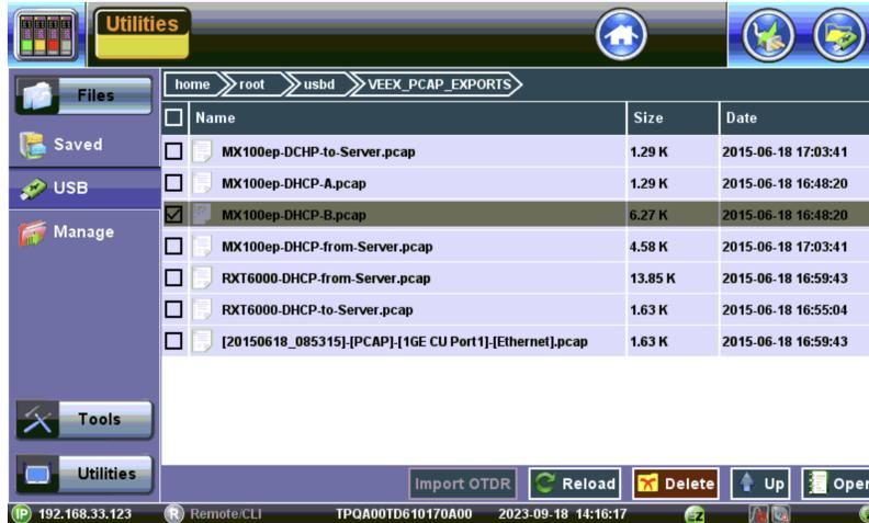
The File Manager (**Files > USB**) provides basic USB memory stick management tools to browse and manage files without the need of a PC. If needed, use the micro-B USB to USB-A adapter to connect to the USB memory stick.
