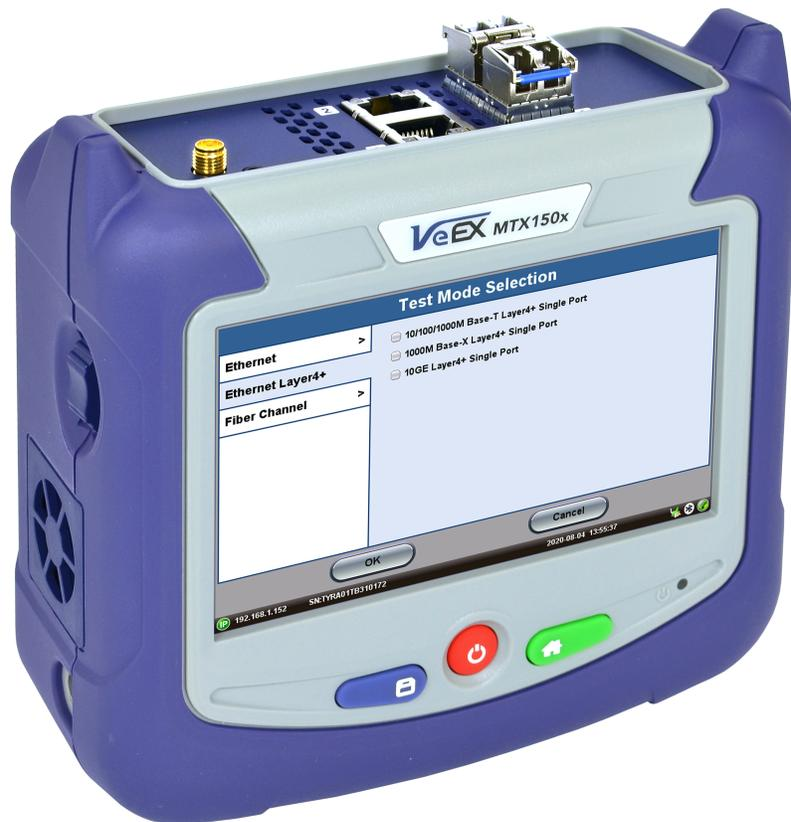
To power on the test set, press
