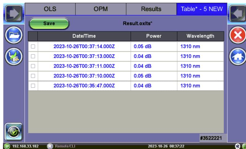
3. To permanently save the fiber record locally, select the record(s) and press **Save**. The **Result saving** screen appears. The filename will default to the date/time stamp unless a specific file name is entered.
